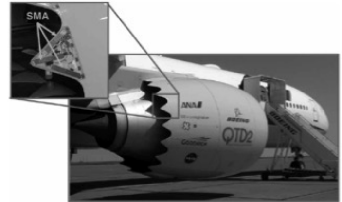
Chevrons for Noise Reduction/Fuel efficiency
