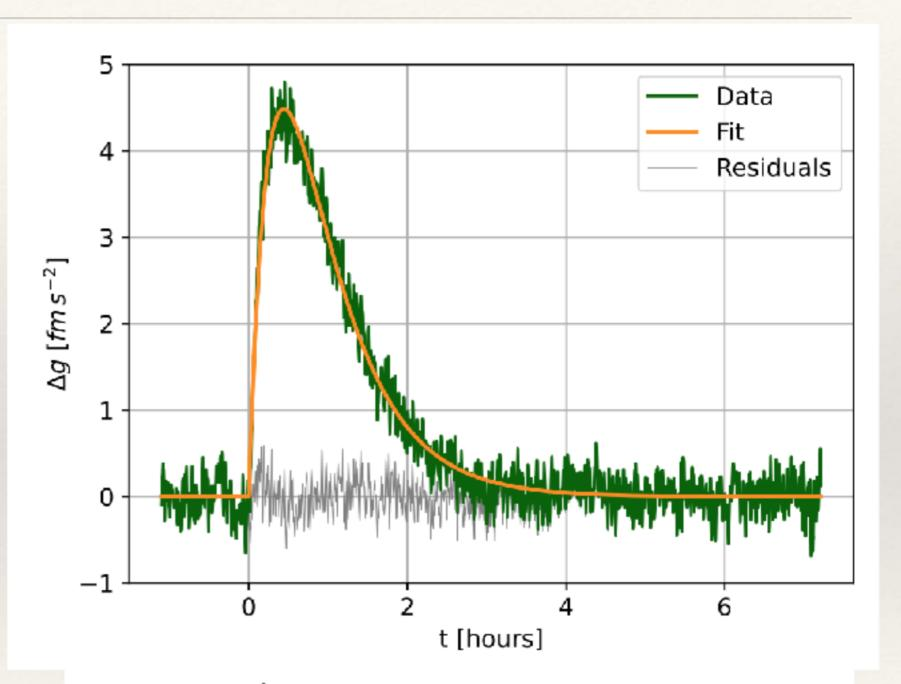
$$h_1(t) = \frac{\Delta v}{\tau^2} t' e^{-t'/\tau} \Theta(t'), \quad t' = t - t_0$$
